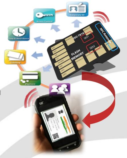
The secure chips of LGM Card can be personalized via a standard ISO7816 contacts placed on the surface of the LGM Card. This enables to use current personalization machines
